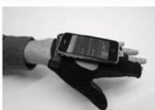
Fig. 1. iPhone wireless accelerometer application for characterizing Parkinson's disease tremor.
