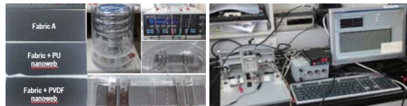
Fig. 1 Setup for evaluating the basic performance of two types of pressure sensors (left: piezo-capacitive, right: piezo-electric)
