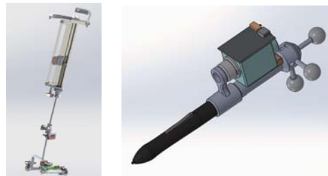
Fig. 2. 3D model of link-type master system (left) and pen-type master system (right)
