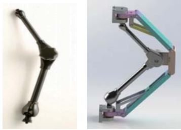
Fig 3. Commercial ball joint links (Left) [3] and 3D design of the passive positioning arm (Right)
