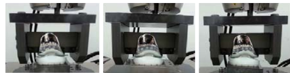
Fig. 1. Test sets-up of contact analysis in varus(left), neutral(middle), and valgus stance(right)
