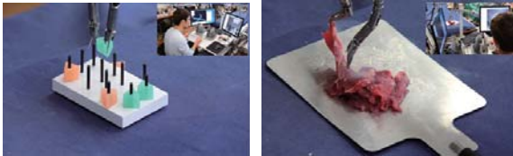
Fig. 7. Dry-Lab test of SPS robot platform: Block transfer (left), Galvanocautery test (right)
