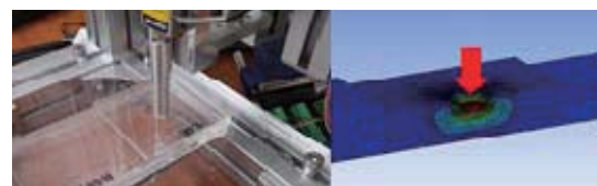
Fig. 1. Indentation test (left) and FEM simulation (right)
