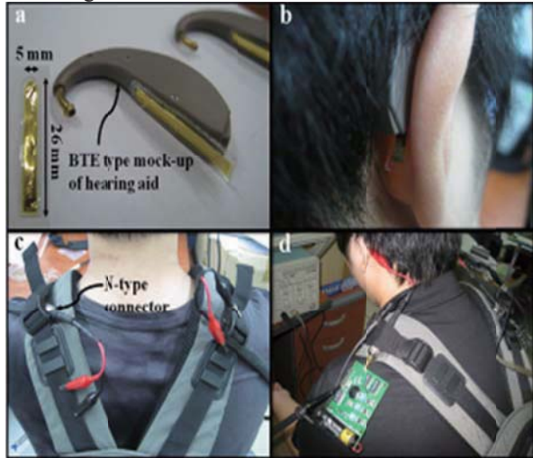
Fig. 2. Preparation for evaluation of PI-PDMS electrodes. (a) PI-PDMS electrodes for binaural hearing aids. (b) attaching electrodes on the retro auricular region after being fixed on the mock-up. (c) connection from NA to N-type connector having forceps. (d) connection of devices for modulation and demodulation with PI-PDMS electrodes for BAN between binaural hearing aids.
