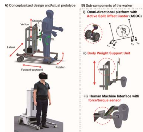
Fig. 1. The design concept and actual prototype of the novel robotic walker for pelvic motion support.
