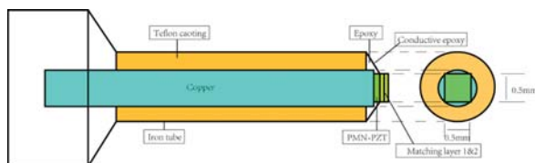
Fig. 1. Structure of the needle hydrophone
