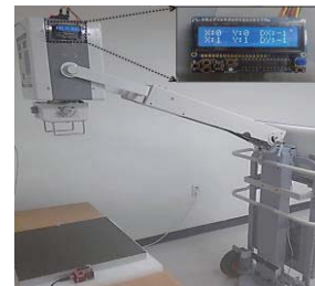
Fig. 2. Portable digital radiography system and display window of LCD monitor on X-ray source
