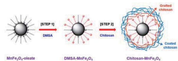
Figure 1 Schematic diagram of synthesis of Chitosan- \text{MnFe}_2\text{O}_4 nanoparticles.
