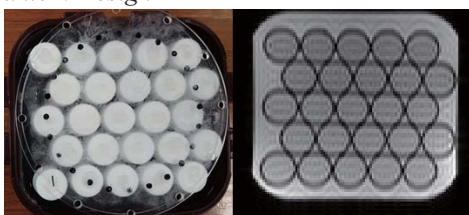
Fig 1. An example of the phantom (left), magnitude image of the phantom (right).
