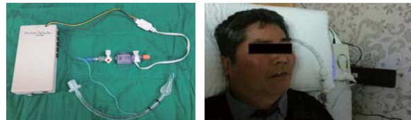
Fig. 1. Alarm system which detect of the dead movement by the pressure variation of a balloon under the pillow of the patient.
