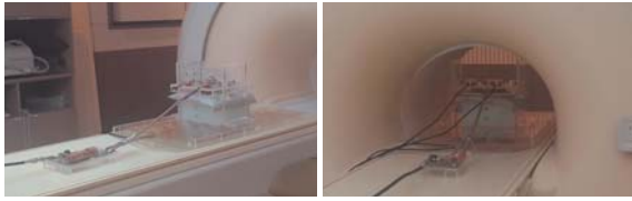
Fig. 2. The RF hyperthermia system installed in the MRI system
