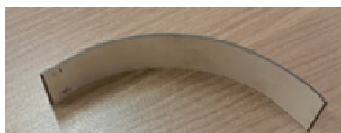
Fig 1. A cylindrical piezoelectric element used to construct a HILFU transducer
