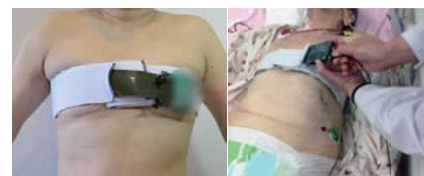
Fig. 4. A wearable EIT and application in ICU
